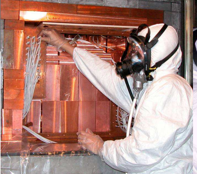
filling the inner Cu box with further shield
